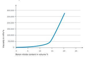
Viscosity measurement by Brookfield DV2-T at 23 °C and 10 RPM in epoxy systems Araldit® casting resin (Carl Roth) spindle 5/7
