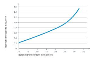
Thermal conductivity measurement via THB 100 in epoxy systems Araldit® casting resin (Carl Roth)
